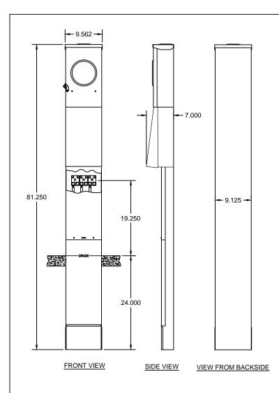
ETL-Certified, NEMA type 3R rainproof enclosure. One piece construction from G90 galvanized steel.
